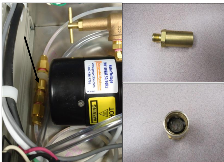
Figure 7.2: Location of Inline Filter in K6300 and buildup of particulates in filter.
