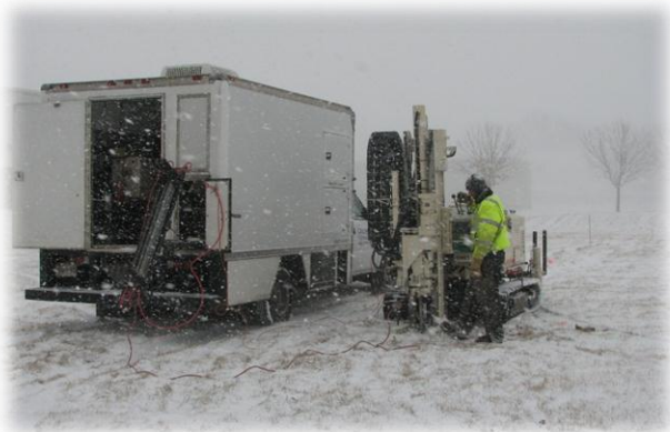
COLUMBIA's direct sensing vehicle during a cold weather MIP investigation at a site in the Midwest
