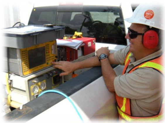
Modular approach configured MIP system on a pickup truck at an industrial site in Mexico
